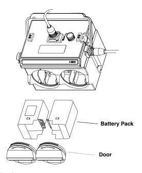
Figure 5-1 Illustration of LTC2191EX Battery Packs
